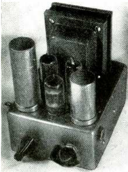
The complete miniature amplifier. The chassis measures only 4 x 5 x 2 inches.
