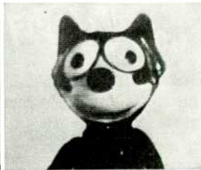
Improved definition is obvious to anyone in this all-electronic 120-line image of Felix—transmitted in the early days of NBC television.
