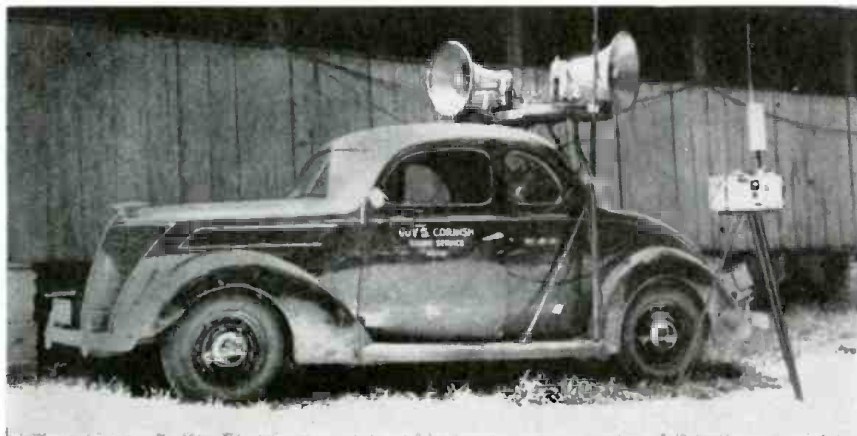
Small transmitter on stand sends voices from rostrum to receiver and amplifier in the car.
