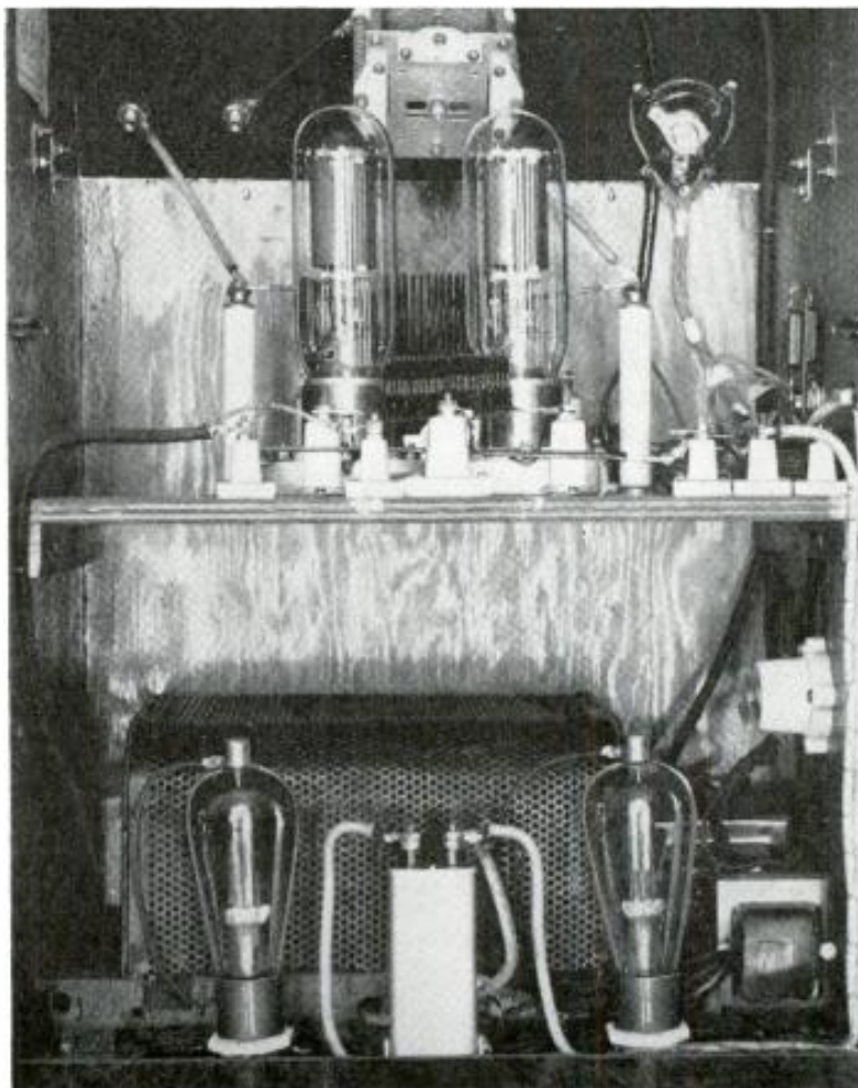
The equipment is mounted on two decks inside the cabinet. R.f. section is on top.
