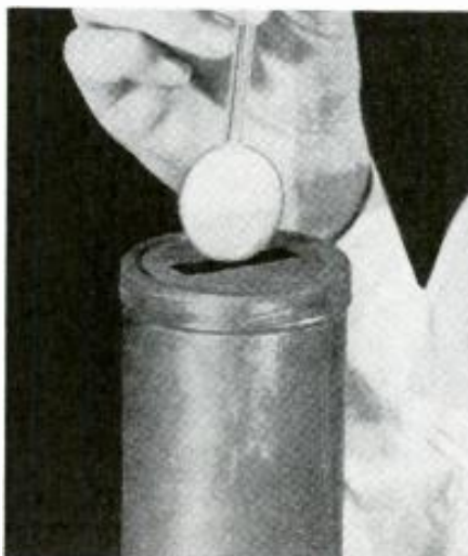
Fig. 7—Lifting electret from Faraday cage. The time required for the charges to reach maximum values is from 2 to 4 months. The growth of charge for one of the author's electrets is shown in Fig. 5. This graph
