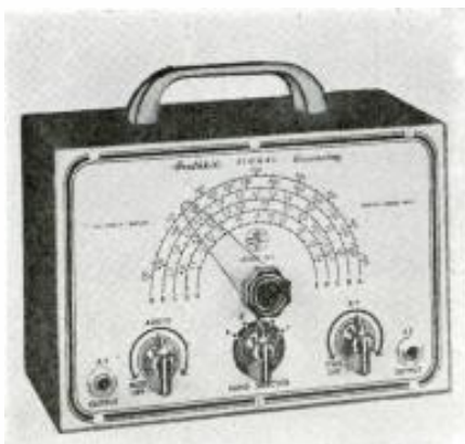
The Heathkit signal generator all assembled.
