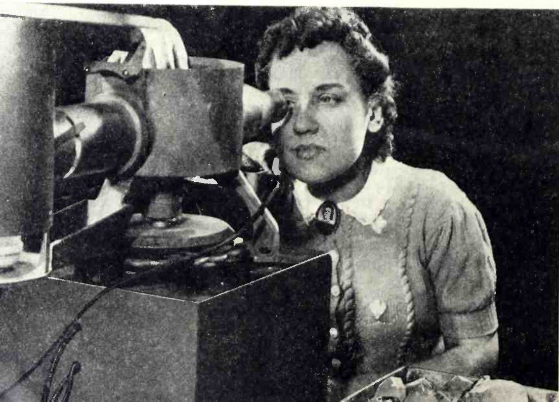
Using a conoscope to determine correct orientation of Z axis.
