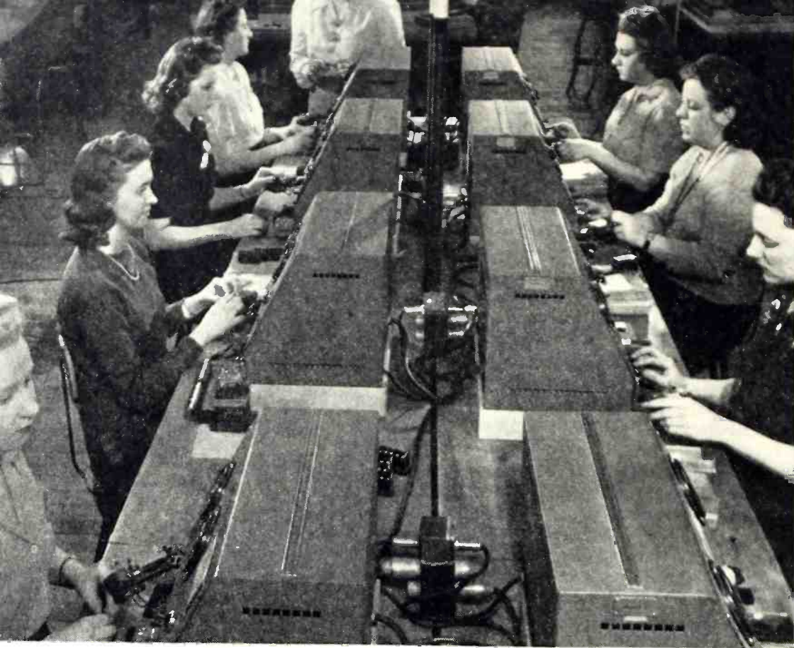
Calibrating and hand-lapping wire-mounted crystal units to final frequency.
