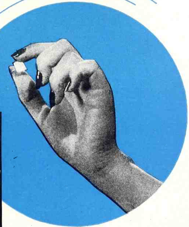
Quartz crystal plate previous to spotting and silver-plating.
