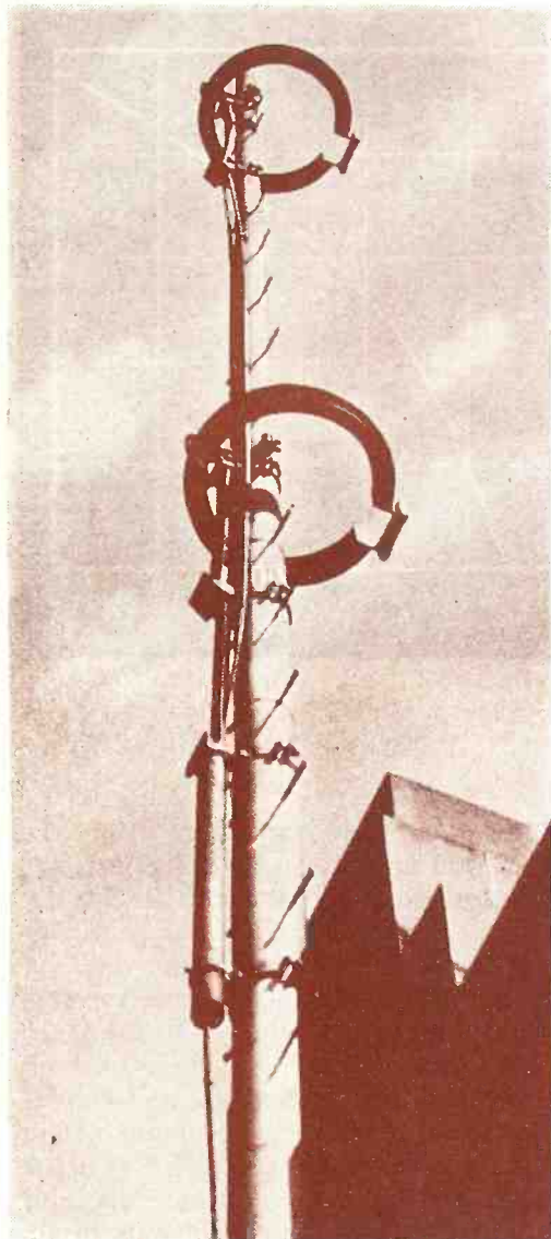
Fig. 2. General Electric two-bay circular antenna as described in Fig. 1.
