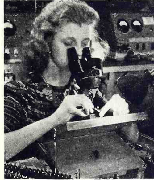
(Left) Soldering of fine lead wires to the electrode surfaces of the crystal. (Center) Close-up of the specially designed soldering machine shown at left. (Right) Inspecting wire-mounted crystal units with the aid of a special microscope.
