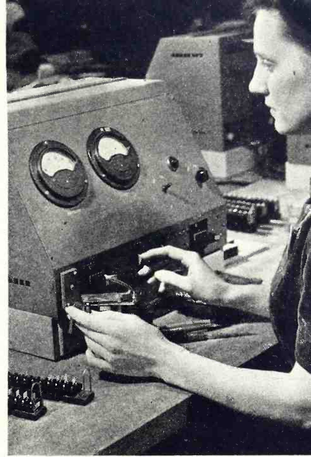
Close-up of calibration and hand lapping to final frequency.
