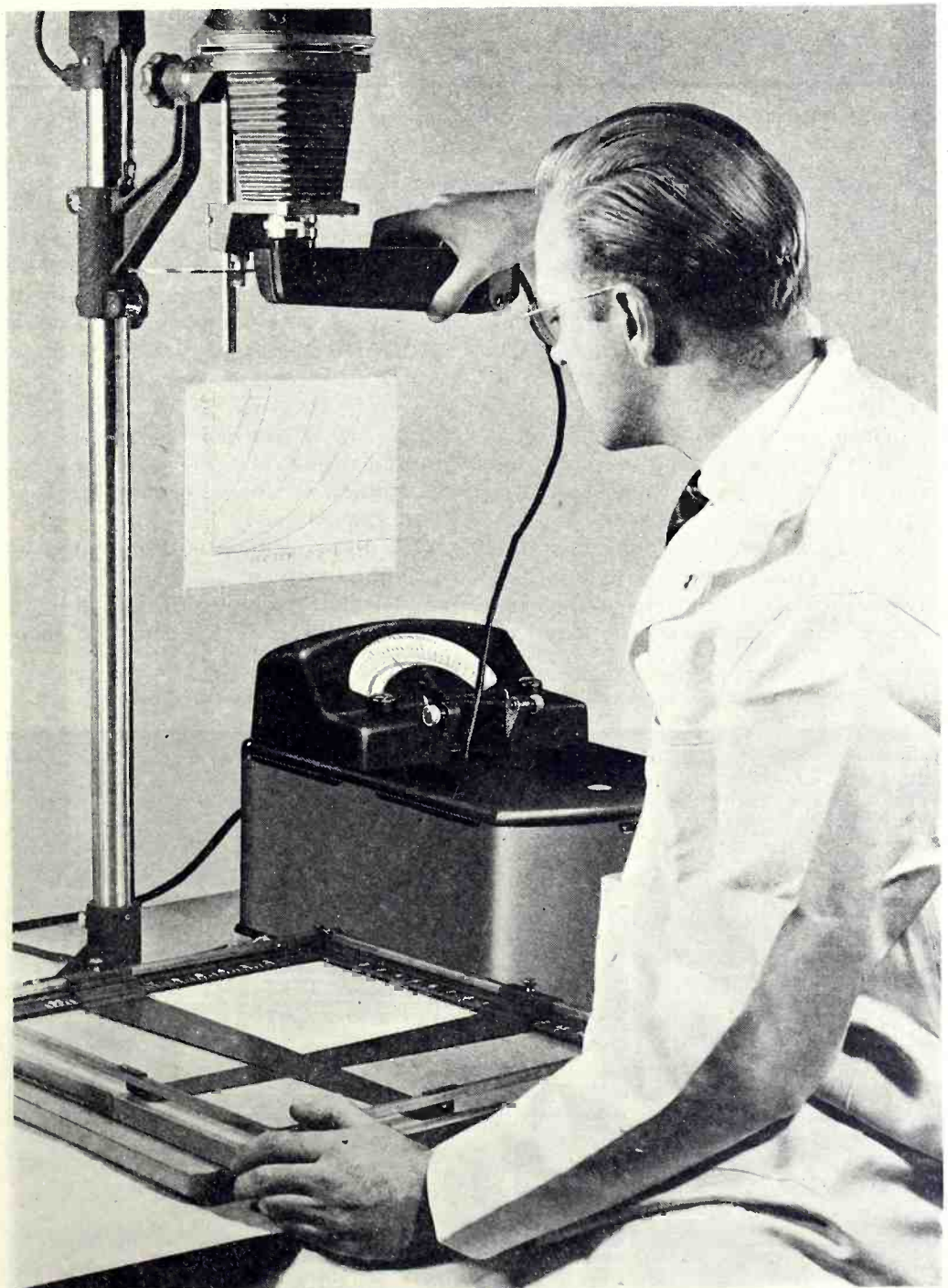
Fig. 1. AnSCO-Sweet Densitometer being used to measure the optical density of a film from which an enlargement is to be prepared.
