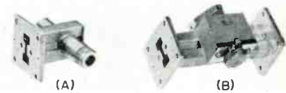
Fig. 4. (A) Ridge wave guide to Type "N" coaxial line transition. (B) Ridge wave guide attenuator, also shown in Fig. 2.
