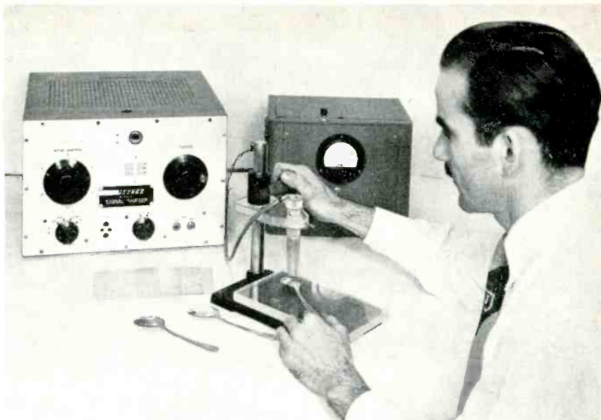
Fig. 1. The Dermatron is useful for measuring thickness of plated coatings on silverware.
