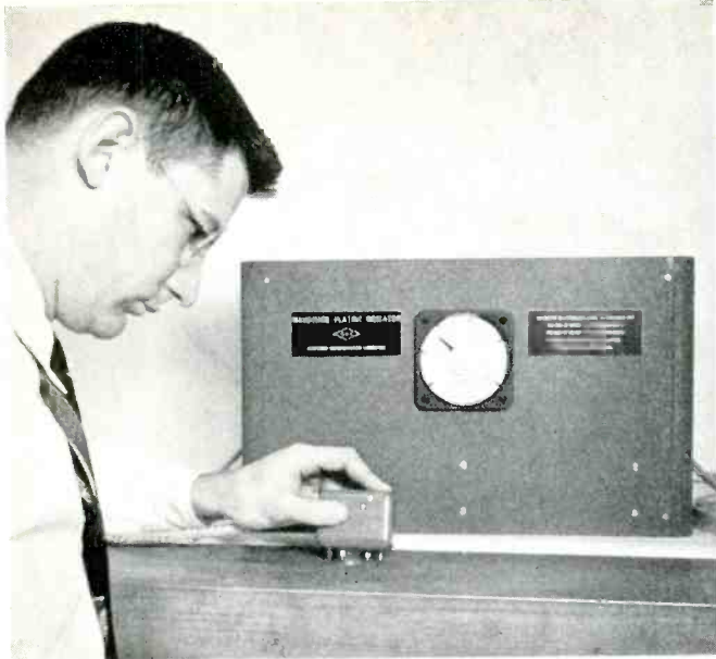
Fig. 3. Wave guide plating indicator uses conductance to determine the thickness of internal plating.
