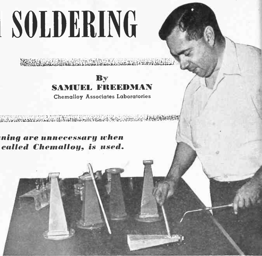
Fig. 1. The author is shown fabricating a wave guide transition by welding together four pieces of aluminum by means of Chemalloy.
