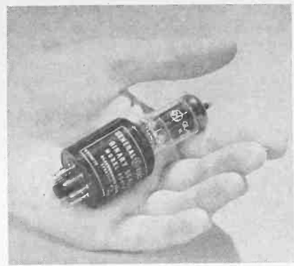
The G-E Type GL-5844 tube for use in moderately high-speed digital computers.
