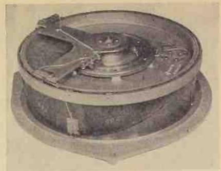
Sine-cosine computer potentiometer manufactured by Electronic Assoc., Inc. for use in computers.
