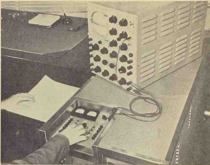
The MADDIDA, made by Northrop Aircraft, Inc. This production model was designed and built for the experimental towing tank of Stevens Institute of Technology. It can be operated by one person, and gives its answer in columns of figures or as plotted curves.
