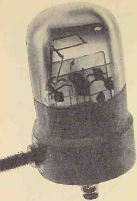
The heart of the accelerometer is this twin diode vacuum tube.
