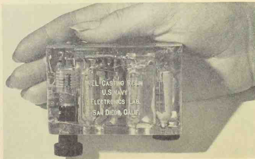
Top view of a complete receiver encased in NEL casting resin.
