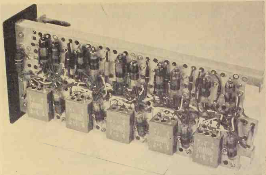
Fig. 3. A plug-in assembly using miniature tubes and parts.
