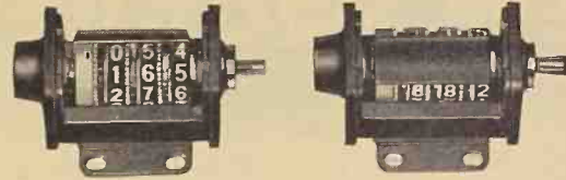
Companion shutter counters used as dual direction indicators. One counter adds while the other subtracts. Shutter blanks out counter which is on negative side of 000.
