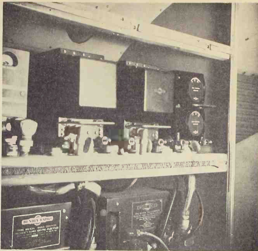
VOR installation in NWA aircraft showing ADF receivers on lower shelf.
