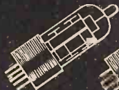
807W Beam Power Amplifier
