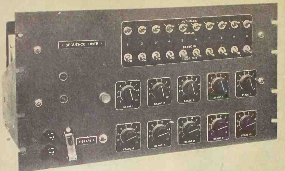
Fig. 2. Front view of the sequence timer control panel.
