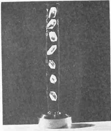
Fig. 5. Arrangement demonstrating growth of several crystals in a single bomb.
