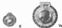
MODELS R AND W DUODIALS Each model available in standard turns-ratios of 10, 15, 25 and 40 to 1. Inner scale indicates angular position of HELIPOT sliding contact, and outer scale the helical turn on which it is located. Can be driven from knob or shaft end. R—2" diameter, exclusive of index. W—4-3/4" diameter, exclusive of index. Features finger hole in knob to speed rotation. — Ask for Bulletins 104 and 114 —
