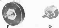
MODELS F AND G PRECISION SINGLE-TURN POTENTIOMETERS Feature both continuous and limited mechanical rotation, with maximum effective electrical rotation. Versatility of designs permit a wide variety of special features. F—3-5/16" dia., 5 watts, electrical rotation 359°—resistances 10 to 100,000 ohms. G—1-5/16" dia., 2 watts, electrical rotation 356°—resistances 5 to 20,000 ohms. — Ask for Bulletin 105 —
