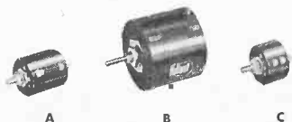
MODELS A, B, & C HELIPOTS A—10 turns, 46" coil, 1-13/16" dia., 5 watts—resistances from 10 to 300,000 ohms. B—15 turns, 140" coil, 3-5/16" dia., 10 watts—resistances from 50 to 500,000 ohms. C—3 turns, 13-1/2" coil, 1-13/16" dia., 3 watts—resistances from 5 to 50,000 ohms. — Ask for Bulletin 104 —
