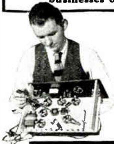
Rear view of 5-tube Screen Grid Tuned Radio frequency set — only one of the many circuits you can build with my parts.
