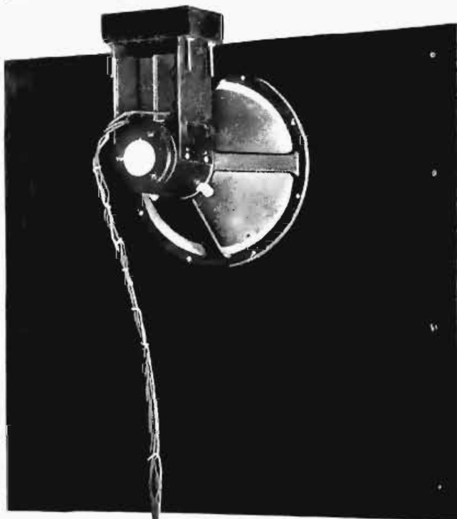
THE Jensen Dynamic Speaker is hung from ceiling of the lower compartment opposite the hole near top of baffle plate.
