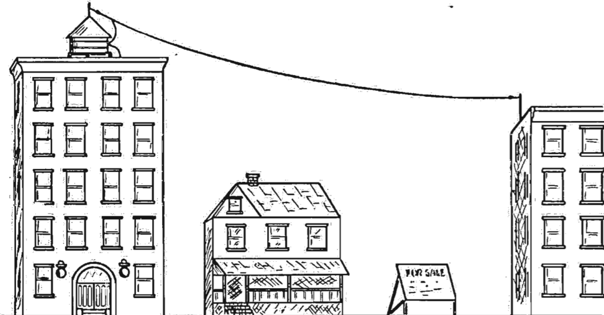
Figure 47—Buildings several lots apart may provide the ideal points for securing the aerial wire
