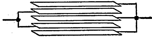
Figure 35—The first step in reducing the size of the two surfaces of a condenser for compactness
