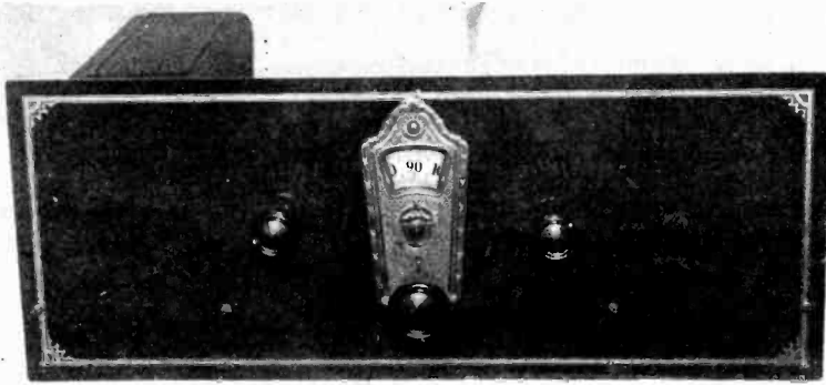
Front panel view of the A. C. Three. Note how the K-111 power pack fits behind the left corner.
