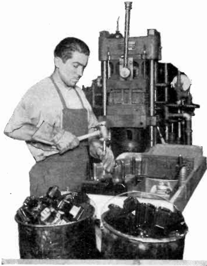
Fig. 2. Moulding bakelite audio frequency transformer cases.
