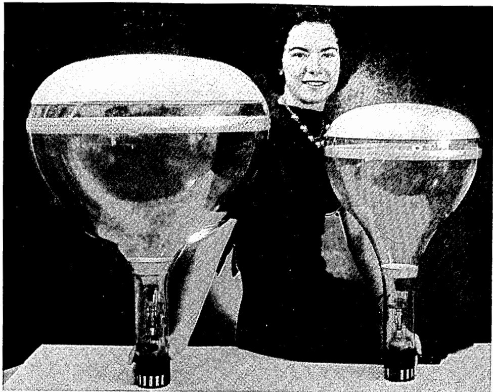
The first 20" cathode ray tube. Photographed in 1938, its size is shown by comparison with the girl and a DuMont 14" tube. The 20" tube is still in daily use in the home receiver of Dr. Thomas T. Goldsmith even after eleven years of use.
