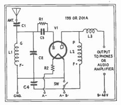
Fig. 43. Grand "Sun" Short-Wave Tuner. A simple circuit arrangement for the beginner. A good design for "breadboard" construction.
