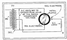
Fig. 70, above. An Electrolytic-Condenser Rectifier. A novel circuit of new design. The output of a unit of this type is limited by the characteristics of the electrolytic condenser. The voltage divider is indicated as "D.C. load." This arrangement is still in the experimental development stage.
