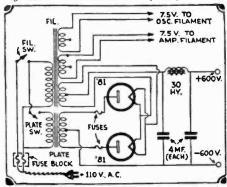
Fig. 98D. Transmitter. Power supply unit.
