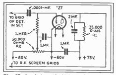
Fig. 87. An Automatic Volume Control Connection. A popular circuit arrangement.
