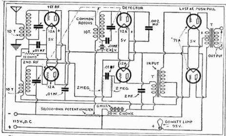
Fig. 11. Grimes "New Yorker" 110-Volt D.C. Receiver. Series-parallel filaments.
