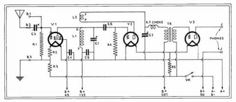
Fig. 38. Short-Wave Screen-Grid "Craft-Box" Set. One R.F., one A.F. stage.
