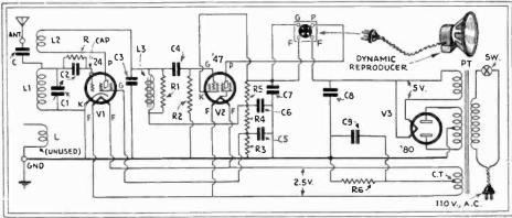
Fig. 2. The Radio-Craft A.C. "Pentode Portable." A Gen-Win 3-circuit tuner is used. The dynamic's field coil is the total filter inductance. Unit L3, 200 hy. or more. Fine experimental, regenerative circuit.
