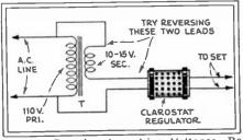
Fig. 84. Boosting Low Line Voltages. Reversing "sec." leads lowers line potential.
