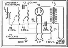
Fig. 78. A Home-Telegraph and Phone Set. With one at either end of the line, 2-way code and voice conversation are possible.
