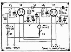
Fig. 98B. Transmitter. Frequency doubler.
