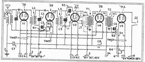
Fig. 12B. Circuit followed in electrifying the Freshman "Masterpiece," Fig. 12A, and other sets of similar design. "Electric" tubes are used as V1 to V5. A type '27 as V3 reduces hum; grid suppressors at X prevent "whistles." Resistor R may improve the operation.
