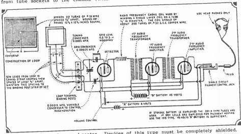
Fig. 72. An Interference Locator. Devices of this type must be completely shielded.
