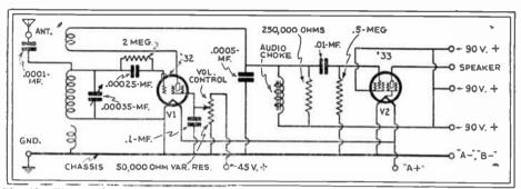
Fig. 16. The Radio-Craft "Pentode Portable"—Battery Model. An improved version of a sensitive, small-space receiver. Regeneration is smoothly controlled by the variable resistor.
