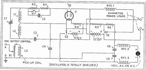
Fig. 79A. A 90-to-1,500 Kc. "Harmonic" Service Oscillator. This instrument is adaptable to 110V. power lines, A.C. or D.C. and also battery operation. Fuse the power leads.
