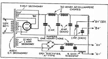
Power pack for the modern, Simple All-Wave Set. Fig. 35B.
