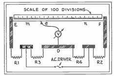
Fig. 97B. Wheatstone Bridge. Meter-rule.
