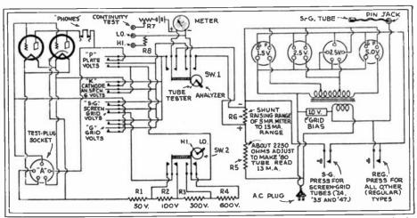
Fig. 101. A Set Analyzer and Tube-Tester. Contains a tube tester, phone-test, continuity tester, pre-heater, ohmmeter, and set analyzer. As designed, it tests all the older tubes without recourse to adapters. Only one meter, 0-5 ma., is needed in this test instrument.
