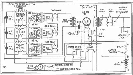
Fig. 81A. A Carbon-Mike Mixing Panel. Accurate matching is obtained by "pads."
