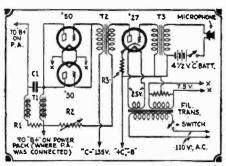
Fig. 98C. Transmitter. Modulator unit.
