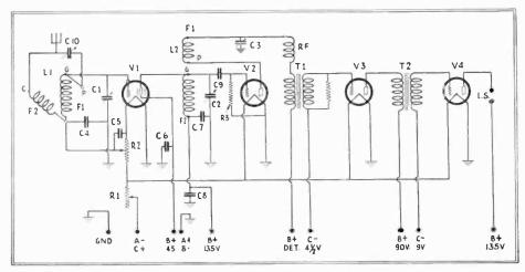
Fig. 48. The Pilot "Super-Wasp" Receiver. A complete receiver capable of reception from distant stations and at "loud speaker volume," so called. A very effective short-wave set.
