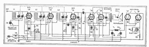
Fig. 7. A Modern A.C.-D.C. Pentode Portable Receiver. Two type '37 tubes, with the elements in parallel, furnish adequate rectification on A.C. circuits; on D.C. they act merely as a series resistance. Tubes V1 and V2 are variable-mu R.F. pentodes. Use no ground.
