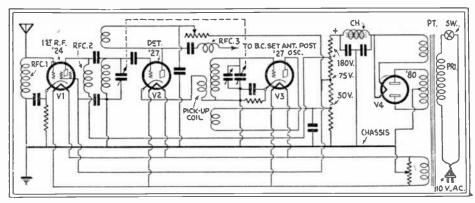
Fig. 54. The Walker "Model 4" Short-Wave Converter. A self-powered instrument.
