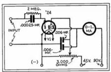
Fig. 91. A Dynatron Vacuum-Tube Voltmeter. Ultra-sensitive, this instrument will indicate 0.2-ma. with an input of only .05-volt, A.C. or D.C. A useful test device.
