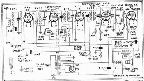
Fig. 8. An Ultra-Modern, Wunderlich-Tube, A.C. Superheterodyne. Tube V2 combines oscillator and first-detector: V4, A.V.C. and second-detector. This set is the Revere Model K2 chassis; the I.F. is 175 kc. Tube V4 is a "coplanar-grid" type Wunderlich "A" or "B."
