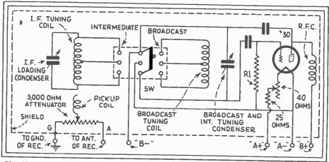
Fig. 85A. A 550-1,500 and 175 Kc. Service Oscillator. Resistor R1 is tone control.
