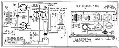
Fig. 66A, left; B, right. A 110-V., D.C. Audio Power Unit. At B, the parts layout.
