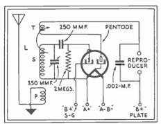
Fig. 14. A 1-Tube Pentode Receiver. For broadcast wavelengths, the grid-leak and grid-condenser may have the usual value, respectively, of about 2 megs. and .00025-mf.; for short-wave reception, over 3 megs. and below .00015 mf. A standard 3-circuit tuner and tuning condenser are used in this setup. Although a battery-type tube is shown, considerably greater output would be obtained from an A.C. tube. The plate voltage will depend on the individual tube.
