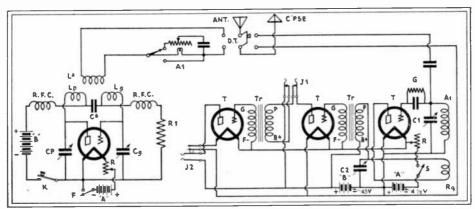
Fig. 74. A Complete Portable Transmitter-Receiver. Transmitter is a "Split-Colpitts."
