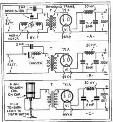
Fig. 95. Experimental D.C./A.C. Converters.
