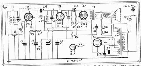
Fig. 9. A Variable-Mu, Screen-Grid and Pentode "3-Tube" Set. A Wal-Tone receiver.
