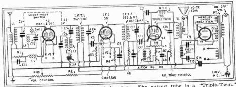
Fig. 10, The Mathews "3-Tube" Superheterodyne. The output tube is a "Triple-Twin." Coils L2 and L3 are inductively coupled. This is an extremely novel circuit arrangement.
