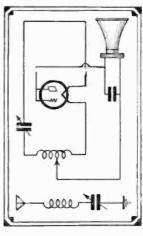
Fig. 34. A Batteryless Tube-Type Receiver. The '71A filament receives its power from the broadcast station, which must be a high power local. The secondary coil is 3% in in diameter and 2% in. long; No. 22 D.C.C. wire; primary, (wound with bell wire), and condenser, experimental. Tuning condenser, 0005-mf.; the speaker bypass, 0.25-mf.
