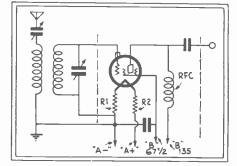
Fig. 79B. Harmonic Oscillator. Graph. Dial "difference" indicates the harmonic in use.
