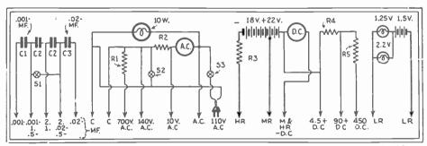
Fig. 92. An Inexpensive Test Panel. The wiring is simple, and the beginner should experience no difficulty with this design. May be used as an ohmmeter, continuity tester, capacity meter, and to read A.C. and D.C. voltages within the ranges indicated—and higher, if so designed. Arrowheads indicate tip-jacks. Condensers C2, 1 mf., each.
