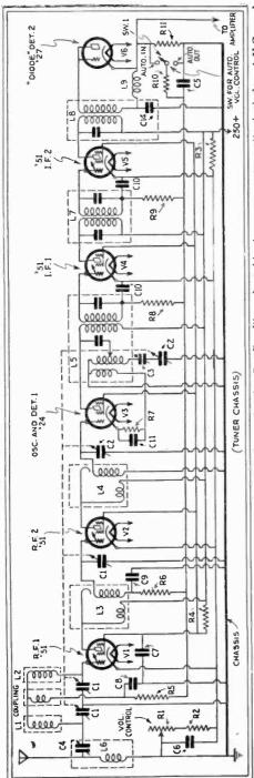
A.V.C. and is a diode. A Modern Superheterodyne Tuner-Chassis-The Super-Da-lite-R. Readily adaptable to any power unit; includes tion. To reduce cross-talk to minimum, type '51 variable-mu tubes are used in R.F. and I.F. Second-detector V6 band-selection. 33A. ġ
