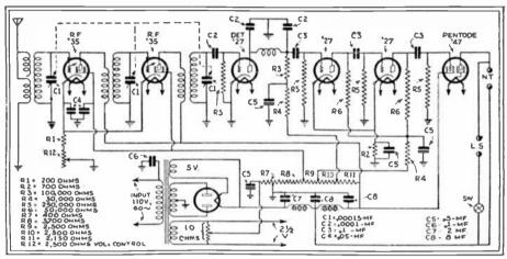
Fig. 57. A Direct-Coupled Television Receiver. Use only accurate, high-watt resistors.
