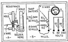
Fig. 94. Increasing A Meter's Range.
