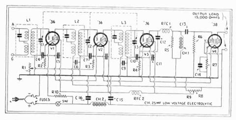
Fig. 5. A 110-volt D.C. Screen-Grid and Pentode 4-Tube Receiver. Note the use of a screen-grid tube as detector V3. Ballast resistor R10 must pass 0.3-amp. and drop to the 25 volts required for the four tubes in series; fortunately, the value is not critical. It is 283 ohms, for a 110-volt line, and 317 at 120 volts. Considerable amplification is obtained.
