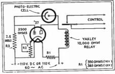
Fig. 76. A P.E.-Tube Relay for A.C. or D.C. Heavy plate current to work relay is due to plate-to-grid-leakage through cell.
