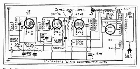
Fig. 6. The "Peter Pan" Model 84 Midget Set. Note the space-saving features: speaker field coil used as filter choke; resistance coupling between detector and power tube. Line switch and volume control are ganged. The output transformer must match V3.
