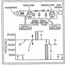
Fig. 96. The Speech Inverter. Above; a skeleton circuit of the method of connections which makes possible "garbled" speech. Below; graphic illustration of the system.
