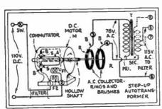
Fig. 75C. D.C. to A.C. Converter. Skeleton view of connections. Transformer T steps up the "R.M.S." output of the motor, M.
