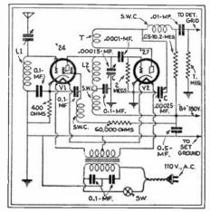
Fig. 53. A Screen-Grid S.W. Adapter.
