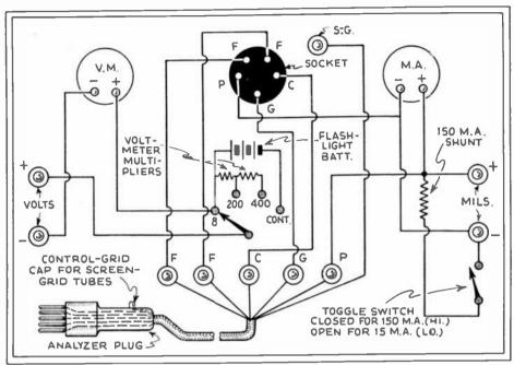
Fig. 90A. A Simple Set Tester. A two-meter instrument of effective pattern.
