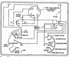
Fig. 86. A Wide-Range A.C.-D.C. Volt-Milliammeter. A general purpose test instrument.
