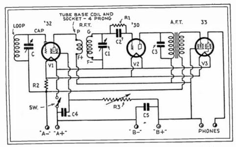
Fig. 93A. A "Treasure" Finder. The receiver; a simple short-wave set for 'phones.
