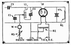
Fig. 98E. Transmitter. Oscillator hookup. When the five component units, A, B, C, D and E are connected together the ensemble is an up-to-date amateur phone and code transmitter—radio station W9DFR.
