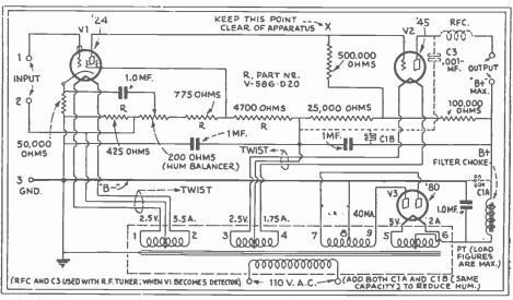
Fig. 67A. Type '45 Direct-Coupled Audio Amplifier. Fidelity is exceptionally good.
