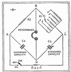
Fig. 97E. Wheatstone Bridge. Capacity.
