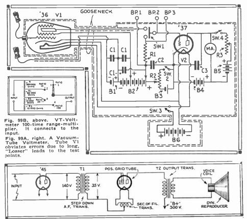
Fig. 100. "Class B Tube" Amplifier. The tube is a "46," designed to operate with zero plate current, under the "no signal" conditions. Note that transformer T1 steps down the voltage.
