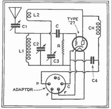
Fig. 52. An A.C. Short-Wave Adapter.
