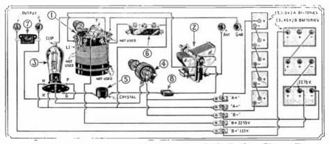
Fig. 1B. Gernsback "Megadyne" 1 tube Loudspeaker Radio Receiver. Picture diagram.
