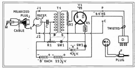
Fig. 65. RCL Public Address Adapter-Unit. Designed to work into an audio amplifier.
