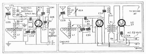
Fig. 47. An "Automatic Tuner" Short-Wave Receiver. By ganging a special variometer L1, and two variable condensers C1, C2A, unique and wide-range tuning is obtained.
