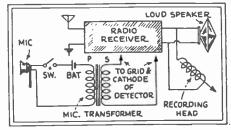
Fig. 62E, left; F, above, Recording. In Fig. 62 we find: A, connections for recording radio programs; B, circuit for recording voice, etc.; C, hookup for "home broadcasting"; D, reproducing recorded voice, etc. These changes may be switch-controlled, as indicated at E. Fundamentally, the circuit is very simple, as shown by the picture arrangement of the parts at F.
