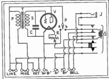
Fig. 77. A Condenser-Mike Pre-Amplifier. The condenser microphone and the pre-amplifier usually are contained in one case.
