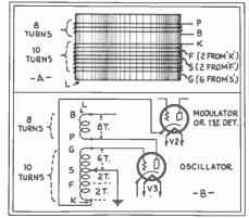
Fig. 55C. Air King Converter. Coil Details. The tickler and secondary windings of L, spaced ½-in., are No. 24 S.S.C. wire, on a tube 1% ins. in diameter.
