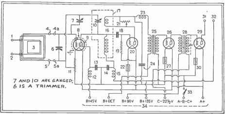
Fig. 17. A Portable Screen-Grid "4" Radio Receiver. A loop antenna is the pickup. If available, an outside antenna may be connected to loop terminals 1 and 2, for increased pickup.
