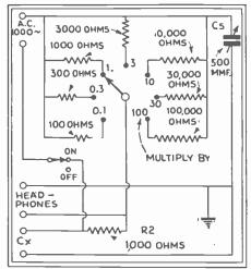
Fig. 97C. Wheatstone Bridge. Capacity.
