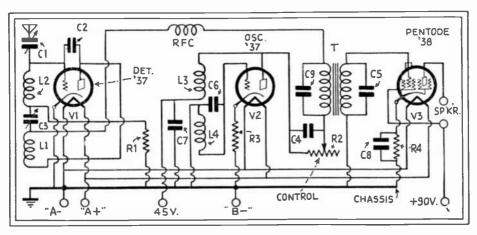
Fig. 39. A 5-Meter Superregenerative Receiver. A "quasi-optical" frequency set.
