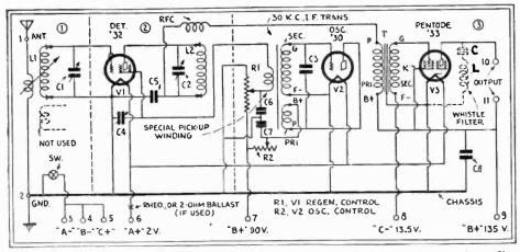
Fig. 46. The Short-Wave "Superregenode"—With 2-Volt or "Dry Cell" Tubes. An ordinary 30-kc. I.F. transformer is used to obtain the super-audible suppressor frequency.
