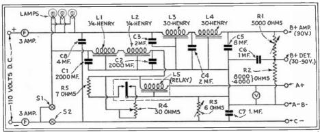
Fig. 69. An "A-B-C" Power Pack for D.C. Lines. Line voltage limits the output potential.
