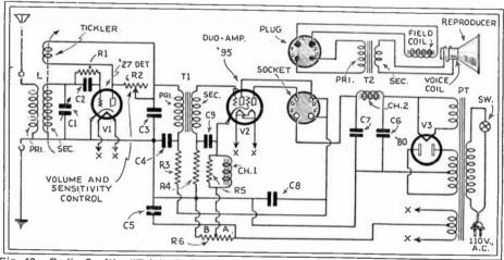
Fig. 18. Radio-Craft's "Triple-Twin" Receiver. Loudspeaker reception is obtained. Experimenters may wish to try circuit arrangements incorporating a "general purpose" pentode as V1.
