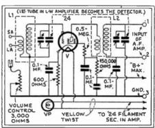
Fig. 15. A Selective Screen-Grid Pre-Amplifier. This is the circuit of connections in the Electrad Loftin-White Type A-224 Tuner, which is designed to be connected to an Electrad Loftin-White Type A-245 direct-coupled A.F. amplifier. The first tube in the amplifier functions as a detector. The advantage of this type of unit is that the amplifier voltages are not disturbed.
