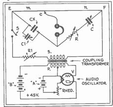
Fig. 97D. Wheatstone Bridge. Tube-type.
