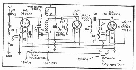
Fig. 35A. A Modern, Simple All-Wave Receiver. Battery or A.C. supply may be used.
