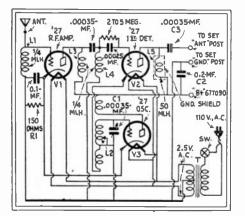
Fig. 55B. The Air-King Short-Wave Converter. Self-powered. A 2.5-volt transformer T supplies the "A" potential for the type '27 tubes used as R.F., det. and oscillator.
