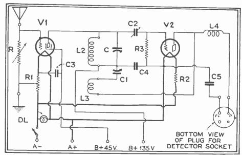
Fig. 49. The Hammarlund Short-Wave Adapter-Receiver. An easily constructed unit.
