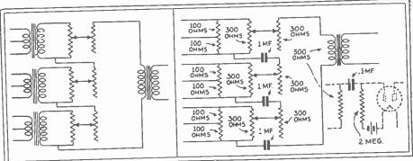
Fig. 81B, left; C, right. Mixing Panel. The 100-ohm resistors in C conserve space.
