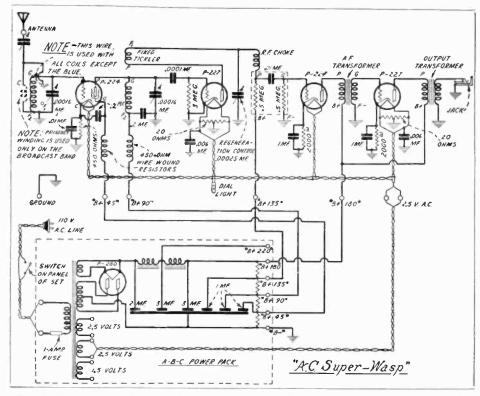
Fig. 40. The Pilot "A.C. Super-Wasp" Short-Wave Set. Four receiver tubes and a rectifier.
