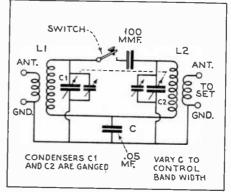
Fig. 88, above. A Band-Selector Unit. By varying the inductive relation of L1 and L2 control of the degree of band selection is obtained. Condenser C and the 100-mmf. unit further control the band selection.
