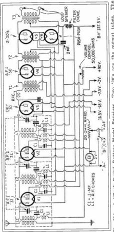
are the output tubes. develops 1.2 watts. '30's 25B A "Push-Push" Battery-Model Receiver. Two Fig. 25A develops 1. watt; the circuit of Fig. Fig. 25A. circuit of
