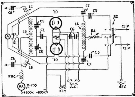
Fig. 98A. An Amateur Short-Wave Transmitter. Connections of the power amplifier.
