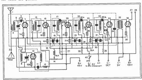
Fig. 59. Cisin "Screen-Grid" Automotive Superheterodyne. Complete details are appended.
