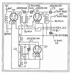
Fig. 55A. The Air King S.-W. Converter. A "Hi-Low" switch shorts 2 turns of L2.
