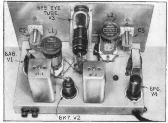
C. Kear view receiver. Flug-in coils amord a simple and emicielli means of changing bands. 01 10.0
