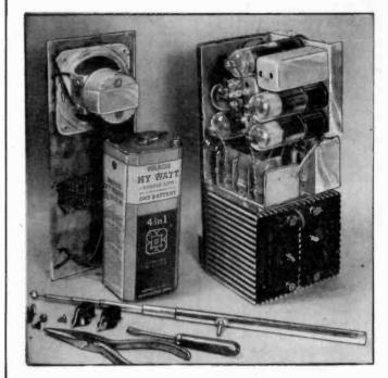
Fig. B. The "innards" of the Lunchbox Portable. One No. 6 drycell will run the set for months. Note the P.-M. dynamic speaker above the cell; and note the telescoping fishpole-type antenna which plugs into the front panel and extends to 45 ins.
