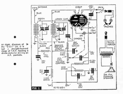
The antenna transformer, T1, is used without the shielding case; but the detector transformer, T2, is left in its metal container and mounted as shown. The remaining parts—resistors, condensers, etc.—can be located in any desired arrangement that lends itself to short connections.
