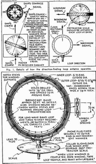
Fig. 2. Detailed specifications on the construction of the loop.
