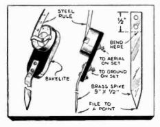
Now take a strip of brass 9 ins. long and <sup>1</sup>/<sub>2</sub>-in. wide. This is bent and bolted to the bakelite as shown in the sketch. A terminal is also provided. In use, the pointed end of the brass strip is pushed into the ground, which should be danipened if it is dry, and the rule extended. The aerial and ground leads are taken right value (to prevent motorboating).
