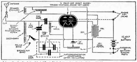
Schematic circuit of the 2-in-j "Card File" Battery Set. If tube V is a ID8GT, connect the screen-grid as shown dotted. Condenser C is a revamped IS-plate Cardwell midget unit. Volume increases with increase of "B" voltage. Use a short aerial or a suitable condenser in series with the aerial.
