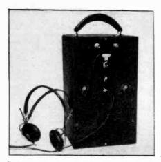
The 2-Tube Superhet., (See Fig. 2 for identification of controls.) with crystal headphones. The tuning range is about 540 to 1,600 kc.
