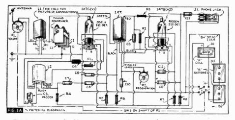
control is then advanced until the circuit is again just oscillating, and the I.F. transformer again adjusted until oscillation ceases. This procedure should be repeated until the primary and secondary are tuned to precisely the same frequency.
