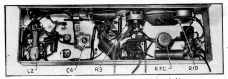
Fig. C. Under-chassis view showing the placement of parts and wiring.
