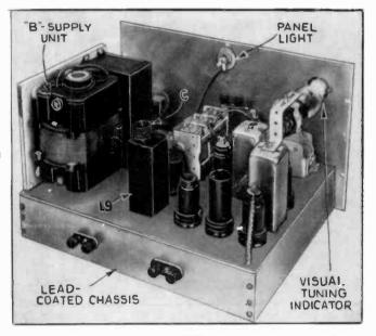
Fig. B. Rear view showing placement of parts and power pack.
