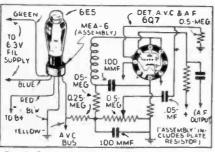
Fig. 5. Connections for the 6E5 "eye" tube, V7.
