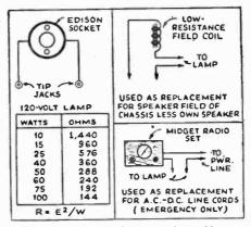
The resistances given in the table are for 120-volt lamps and this data is intended as only approximate. You must experiment to get just the right lamp for the particular application you wish.
