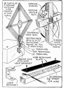
Fig. 2. Details of the collapsible loop.
