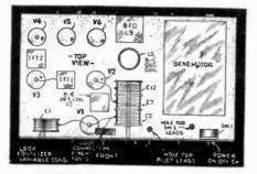
Fig. 2. Layout of parts on the chassis.
