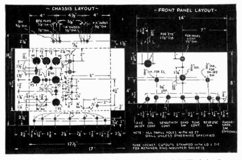
Fig. 4. Physical specifications for making the front panel and chassis for "The Seafarer."
