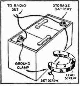
Ground clamp makes good battery terminal.
