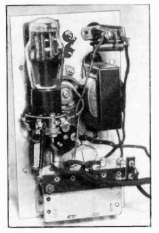
Fig. 8. Internal view of the compact 1-tube set. All parts are mounted behind the top panel of the box and are therefore readlly accessible.
