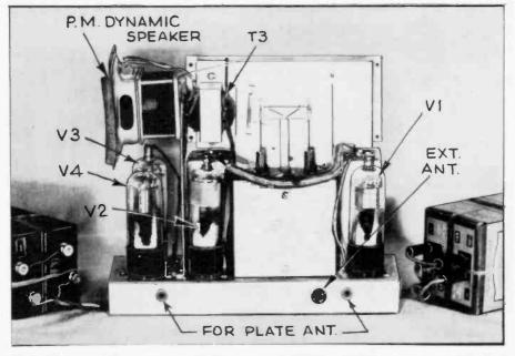
Fig. B. Rear view of the portabe showing the locations of the tubes and other components with respect to the permeability tuner. The antenna plate plugs into the 2 extreme jacks and may be used for local reception. When in the country, away from stations, use a 20-ft. length of wire plugged into the remaining jack.
