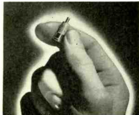
Fig. 3—Typical crystal for converter stage.
