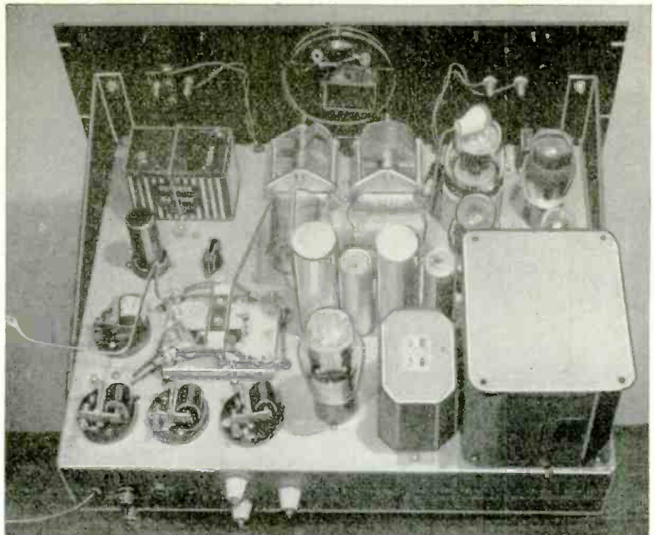
Fig. 2—The power supply is shown at the lower right in the picture. Coils are at center.
