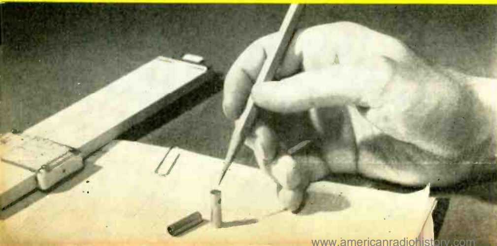
Fig. 1—This photograph shows how small the amplifying unit is. The crystal and the two contacts are enclosed within a tiny cylinder.
