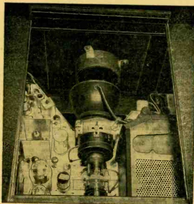
Photo 3—The projection lens and 30-kv tube.
