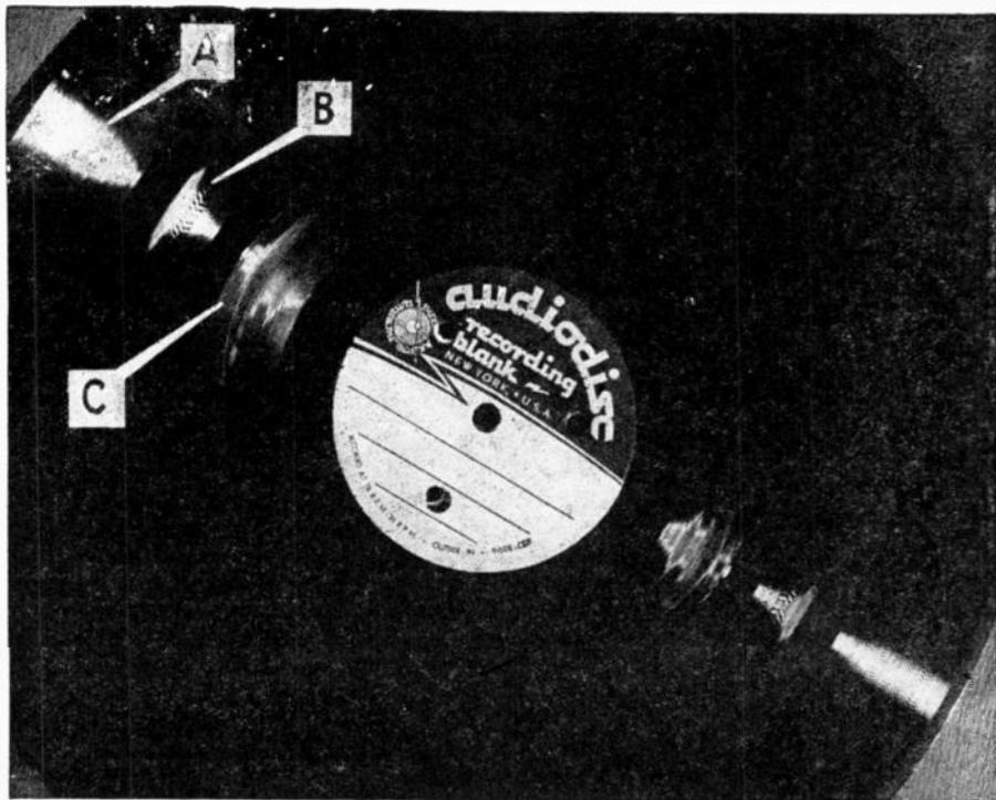
Photo A—A and B are constant-velocity and constant-amplitude patterns respectively. C is an example of bad resonant peaks showing severe distortion caused by over-modulation.
