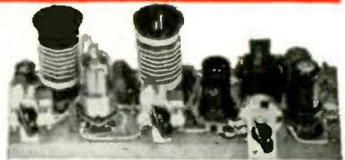
Above: You build this tuned radio stage, regenerative detector and audio amplifier. (Experiment No. 329)
