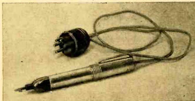
The crystal probe in its small penlite case.
