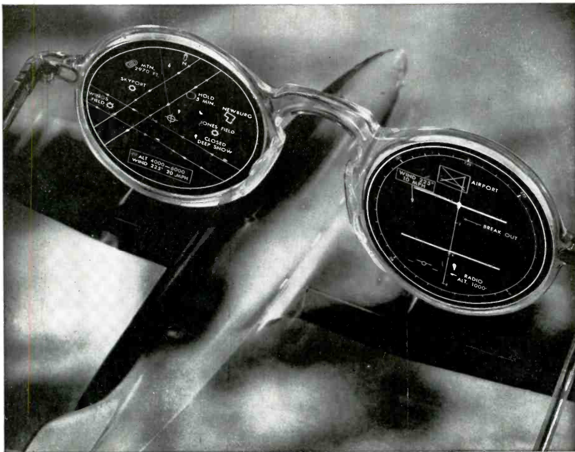
Teleran pictures—air traffic control by radar plus television.
