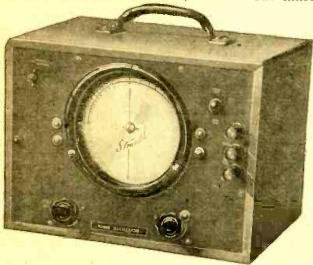
The beat-frequency oscillator is compact and easily carried around.
