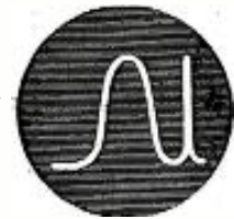
Fig. 4—The single-curve alignment pattern.
