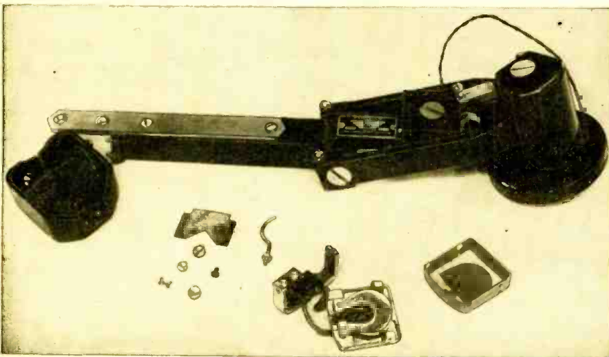
Semi-exploded view of the new pickup, showing jointed arm and the interior pickup head.
