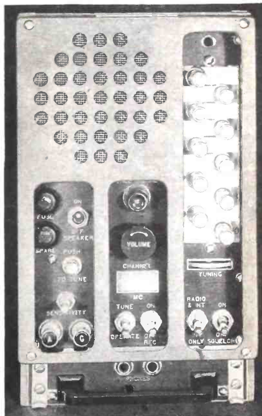
Fig. 2—The BC-603 receiver. Lamp above volume control lights when signals are received.
