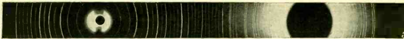
Above, the diffraction pattern for tungsten; on opposite page, that for copper. Line spacing and brightness identifies the material.
