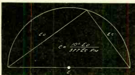
Fig. 9—Meters may be calibrated without recourse to cut-and-try, using the chart above.
