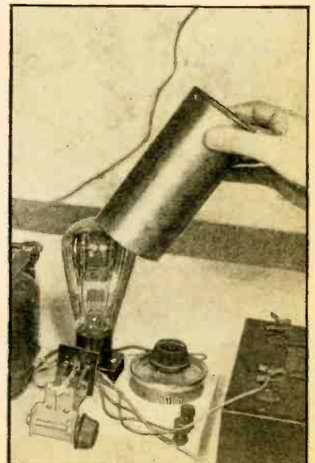
A close-up of the 210 photo-cell circuit with shield off.
