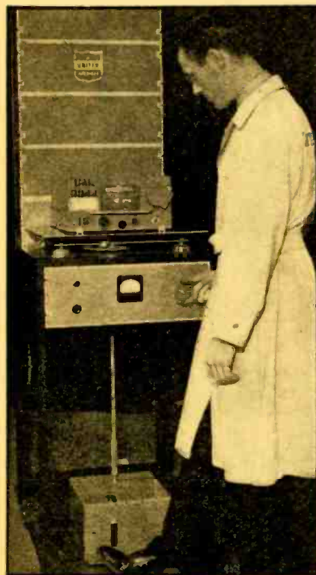
NEW "SHAKE TEST" FOR RADIO: Here is United Air Lines' newly-designed vibration generator for testing aircraft radio equipment under conditions considerably in excess of those encountered in flight.
