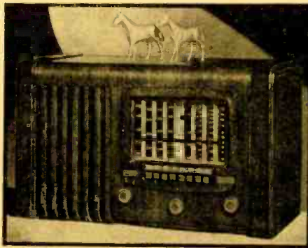
The Pilot Model No. 340 A.C.-D.C. receiver, covering the short wave and broadcast bands.
