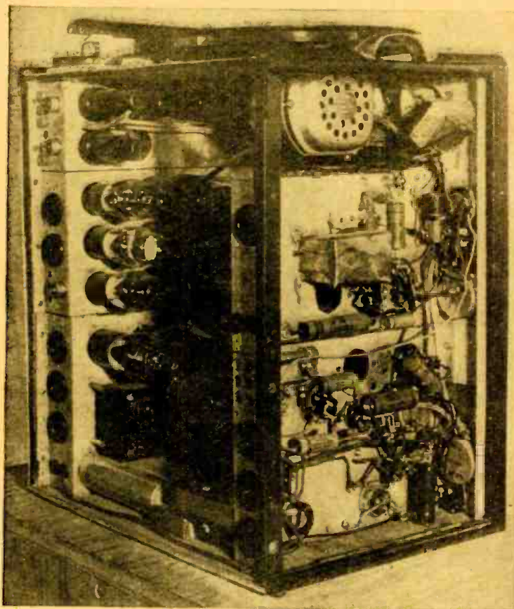
Photo at left shows view of the main chassis array, with amplifiers and phono motor. The sectional unit construction makes repairs a simple matter.
