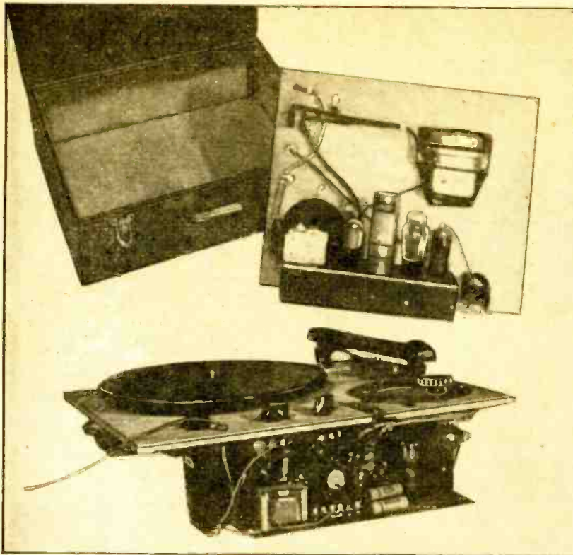
The photos herewith show the phonograph unit as designed and built by Mr. Tait, together with the crystal pickup and volume indicator. An interesting new wireless oscillator is described by the author, which permits records to be played through the receiver without direct connection. It is also possible to feed radio or microphone "pickup" into any receiver.
