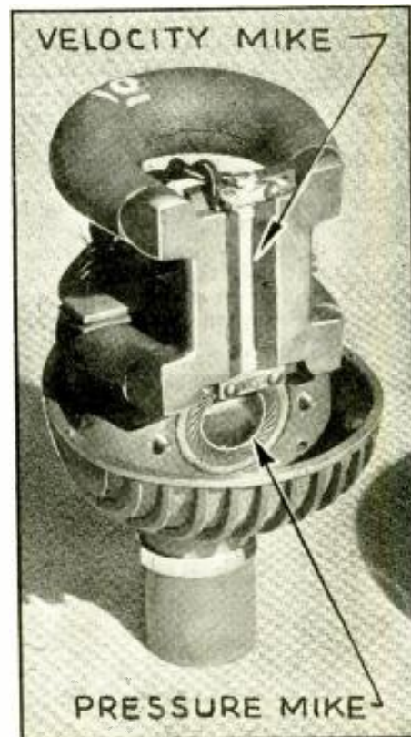
Here's a glimpse inside the Western Electric model 639A Cardioid Microphone. Compare with cross-section at left. Ribbon and dynamic microphones are combined in one compact unit.
