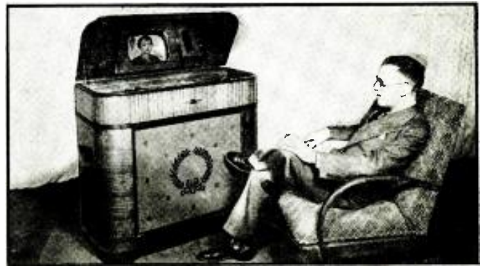
Dr. W. R. G. Baker, chief of G-E's radio & television division management committee, looks pleased with the performance of his dept.'s new model which the co. will offer in limited quantities this Spring. Controls are placed under lid which has inclined mirror for televiewing. (Yes, it's an imitation image we dubbed in for art's sake.—Editor)
