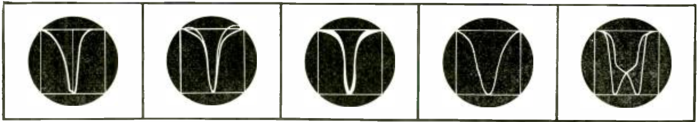
Fig. 4N. Flat-topping due to overloading. Reduce input to receiver. Fig. 4P. Phase distortion in the output circuit. Fig. 4Q. Showing width of the I.F. channel. Fig. 4R. Pattern showing interference being received. Fig. 4S. Uneven curves caused by regeneration.
