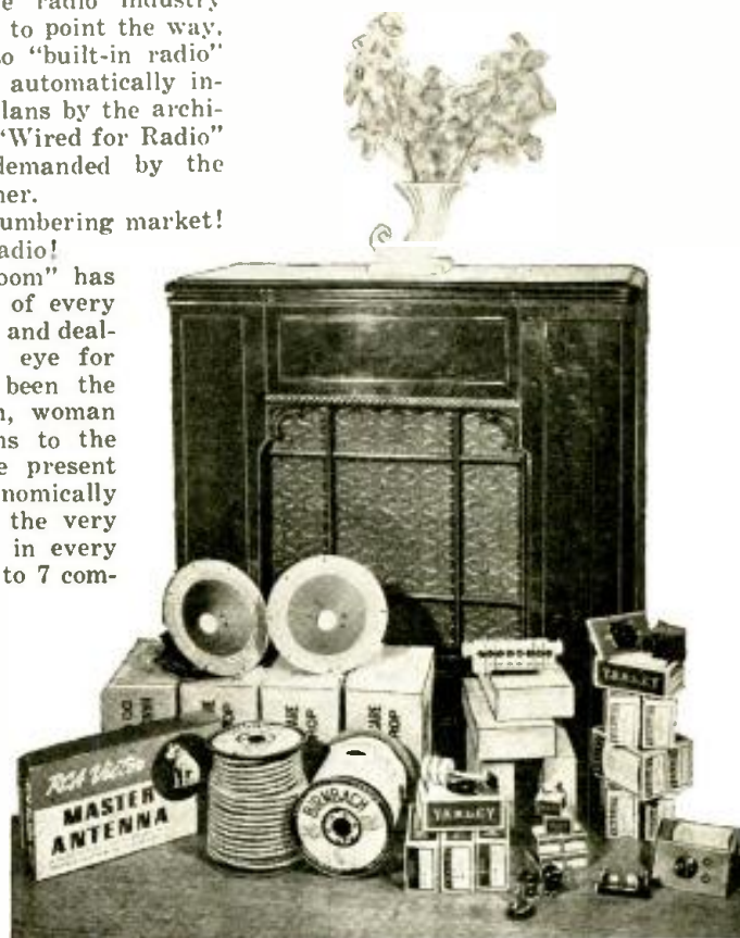
These are the major components of the built-in radio system. In the background is the beautiful RCA-Victor high-fidelity victrola-radio combination model U-130. In front of it are 6 (7 will be used) RCA P.-M. dynamic speakers; 6 Mallory-Yaxley pushbutton switches, multi-contact outlets, pilot light sockets, and combination power and combined "Ant.-Gnd." outlet; Birnbach 7-wire shielded cable; RCA-Victor master antenna; and relay for turning the set on and off, remotely.
