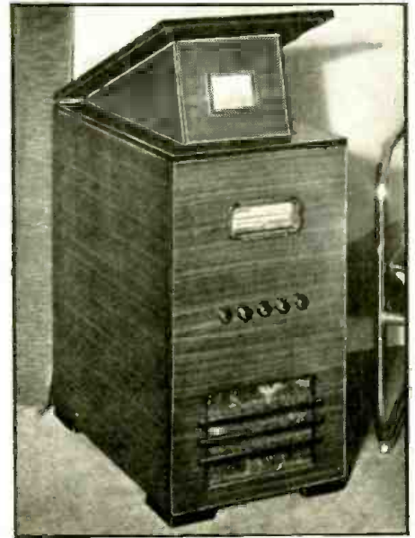
Fig. A. The Garod demonstration television receiver. The tube housing closes down with the lid.
