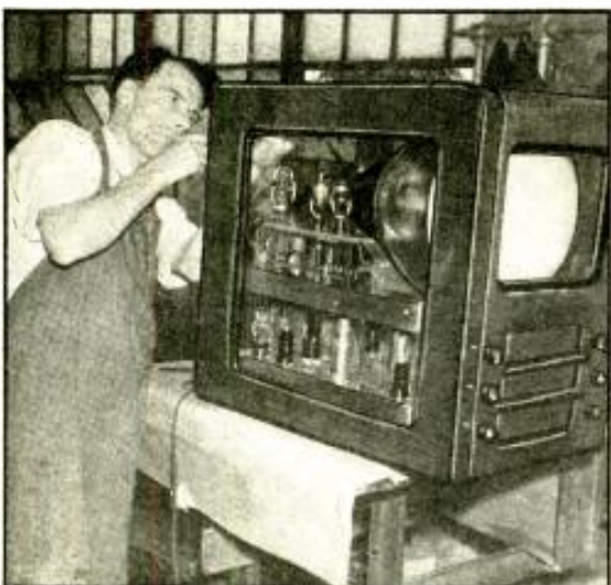
A WORKER IN AN AMERICAN FACTORY CHECKS-UP A . . . "14-INCH" TELEVISION RECEIVER AND ITS HUGE C.-R. TUBE
