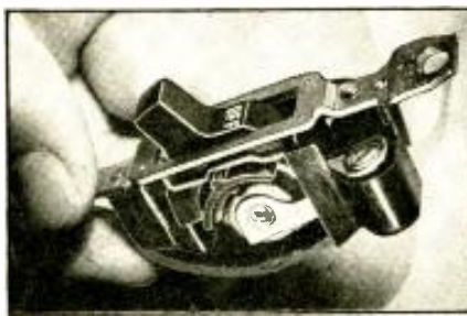
Silent mercury-break toggle switch. (1710)
