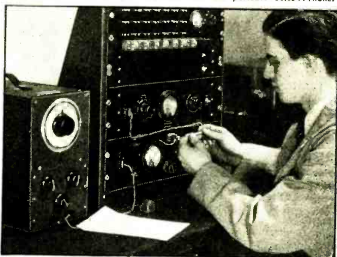
Fig. C. The "intensifier" (electromechanical amplifier) being checked and adjusted against an oscillator and level indicator (decibel meter).
