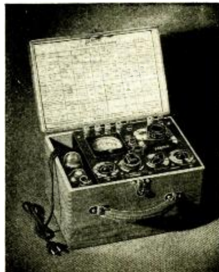
New condenser and resistor bridge. (1676)
