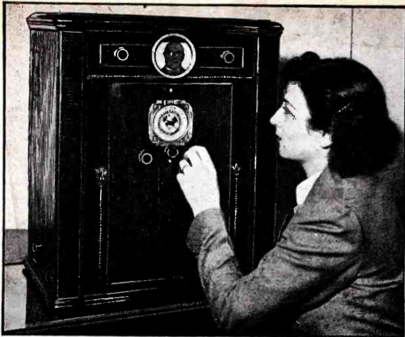
Fig. A. The $125 video receiver; 3-in. tube (image area, 1\frac{1}{4} \times 2\frac{1}{2} ins. wide).
