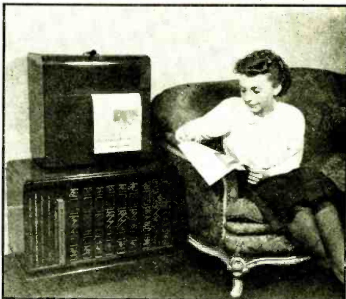
Fig. F. How the RCA home facsimile receiver looks; a time clock turns it on and off.
