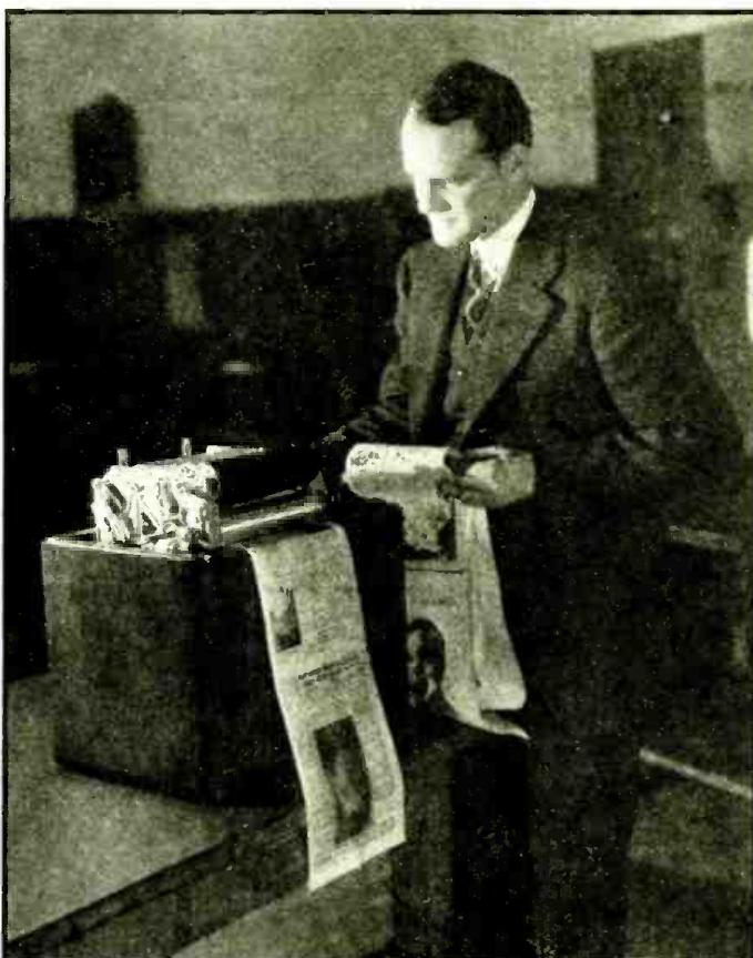
Fig. E. RCA-Victor engineer C. J. Young, developer of RCA's home facsimile system, poses beside his new receiver, which is opened to show its working parts.
