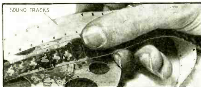
Fig. C. "Wavy"-type groove is indented directly on the surface of the film.
