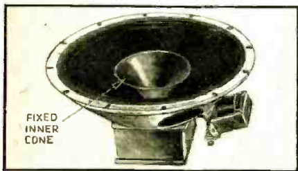
Fig. A. English hi-fi speaker using small, fixed center cone to distribute the "highs".
