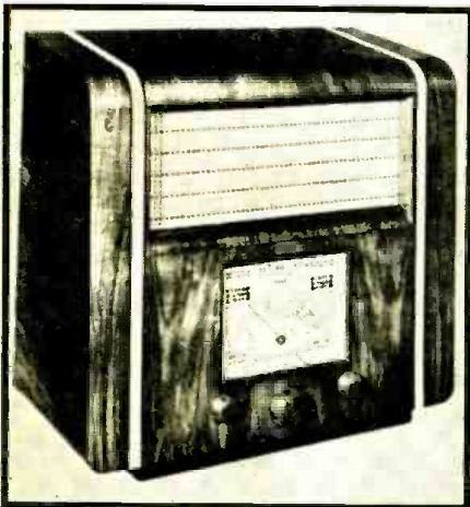
Fig. C. A useful innovation in this British set is the enlargement (by photographic projection) of that portion of the scale to which the dial points.
