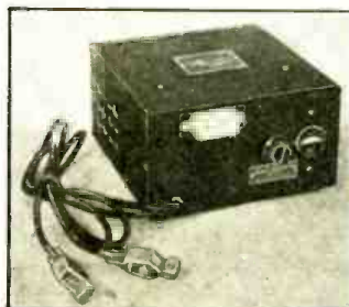
New D.C.-A.C. inverters. (1512)
