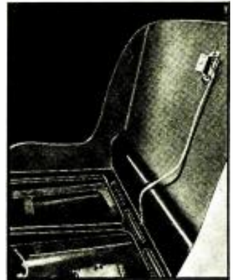
Installing the seat reproducer.
