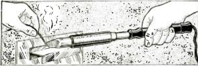
The correct angle to hold the iron is flat to the work.
