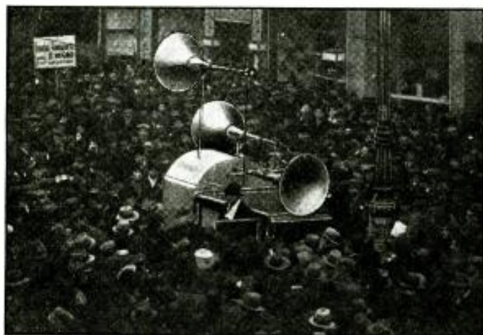
Fig. A. Mobile P.A. using 6 ft. aluminum demountable horns.
