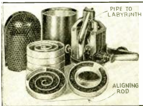
Fig. A. The completely-assembled view, left, of the new directional-type ribbon microphone shows it to be more than 1 ft. long. The lower-half of the case encloses the rod-aligned labyrinth sections (see view at right).
