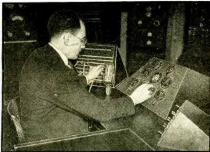
Fig. A. A velocity microphone installed in the Hotel New Yorker high-fidelity system.
