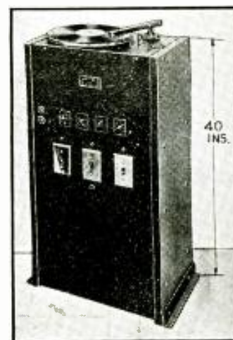
Panel amplifier. This 50-W. set-up will drive 50 dynamics. (1336)
