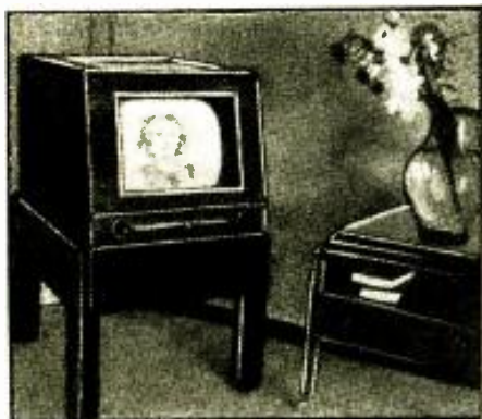
Fig. A. Notice the squat appearance of this television receiver—for seated viewers.
