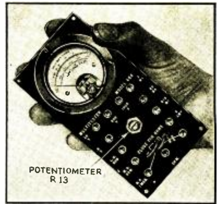
Fig. A. The size and appearance of the tiny volt-meter-ohmmeter-milliammeter-microammeter.
