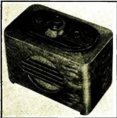
As illustrated and described in RADIO-CRAFT Oct. 1936, pgs. 204 and 205, this set has loudspeaker grilles on 2 sides of the cabinet. Set has a "glowing beam station indicator."
