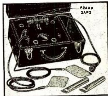
Photo—Diathermy Co. of America Fig. D. A "spark"-type diathermy machine. The wavelength is 18 to 20 meters—diathermic capacity is 1,500 milliamperes. Uses a multi-section gap.
