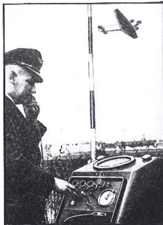
One of the transmitters located on an air-lane which is used for blind flying in Germany.
