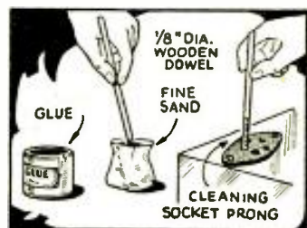
Fig. 12. Socket prong cleaner.
