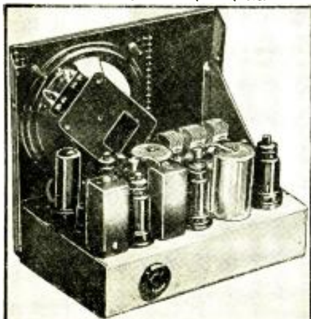
The rear of the receiver chassis showing the compact mounting of tubes, coils, etc.
