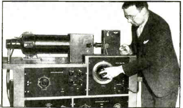
Fig. C. This "analyzer" segregates and records every component in a given sound.
