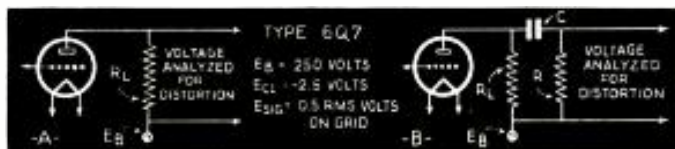
Fig. 1. The 2 circuits used in the tests described. Circuit A is used in obtaining the curve A in Fig. 2, below. Curves B, C and D were derived from circuit B
