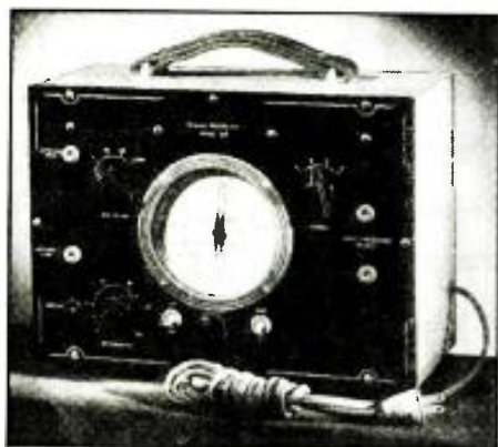
Above, the appearance of an A.C. powered signal generator, especially designed to supply the needs of the Service Man.
